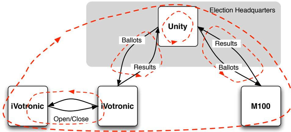
Figure 5: Viral loops through ES&S components
