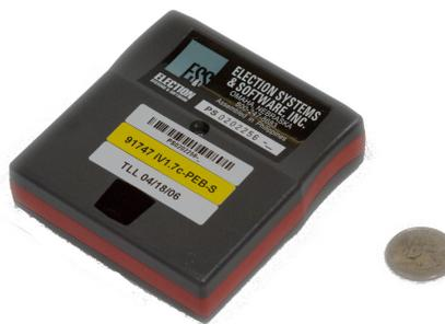
Figure 2: An ES&S “Personalized Electronic Ballot” (PEB) used to transport ballots and results between the iVotronic and Unity.
